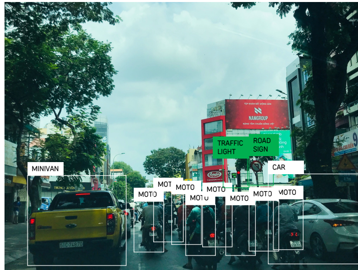
Figure 1.5: This image portrays a road scene in Ho Chi Minh City, Vietnam, with various road objects annotated. It's important to note the presence of numerous potential false sources that could complicate the recognition process, including billboards and vehicles parked on the pavement.
